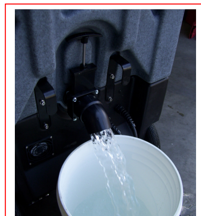
Drain water from Recovery Tank
