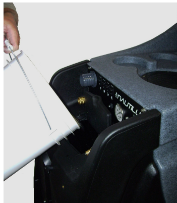
Pour appropriate amount of hot water into solution tank
